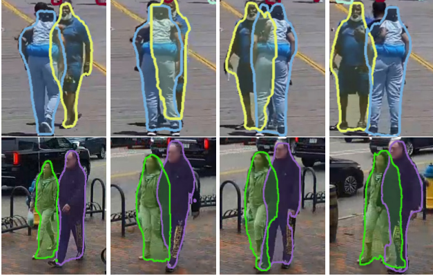
Figure 10. Accurate prediction of amodal segmentation of people when a person passes by another (top) or when they walk occluding throughout the video (bottom). Such representation directly extrapolates to improved tracking of people in generic videos.
