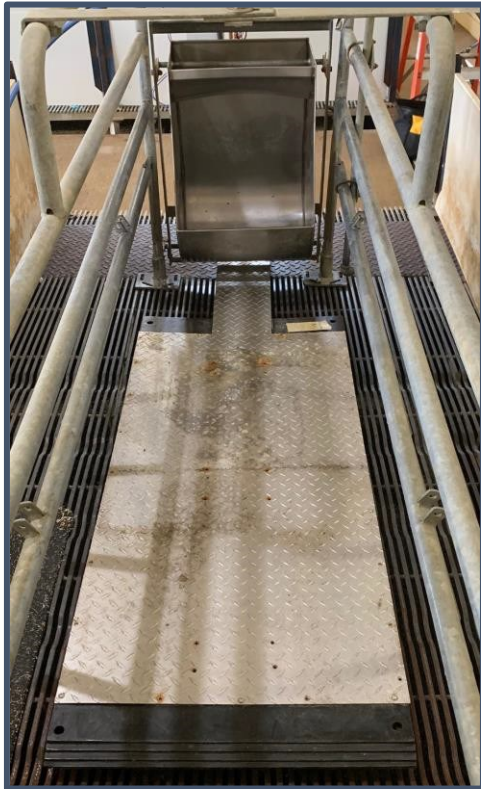
Figure 1 - Purdue Hog Cooling Pad
