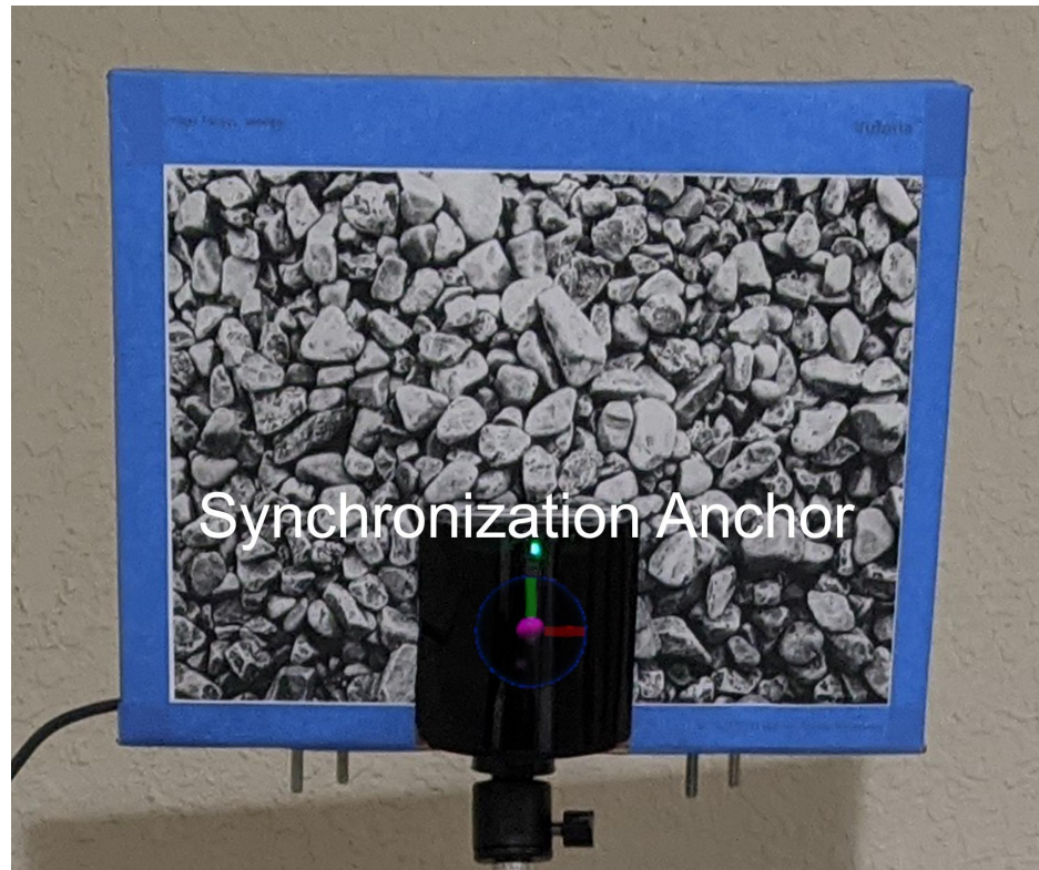
Figure A.1: Vuforia image target mounted on top of Vive-Pro Base Station 2.0, synchronization anchor position adjusted down from the center of the image target to the base station center.
