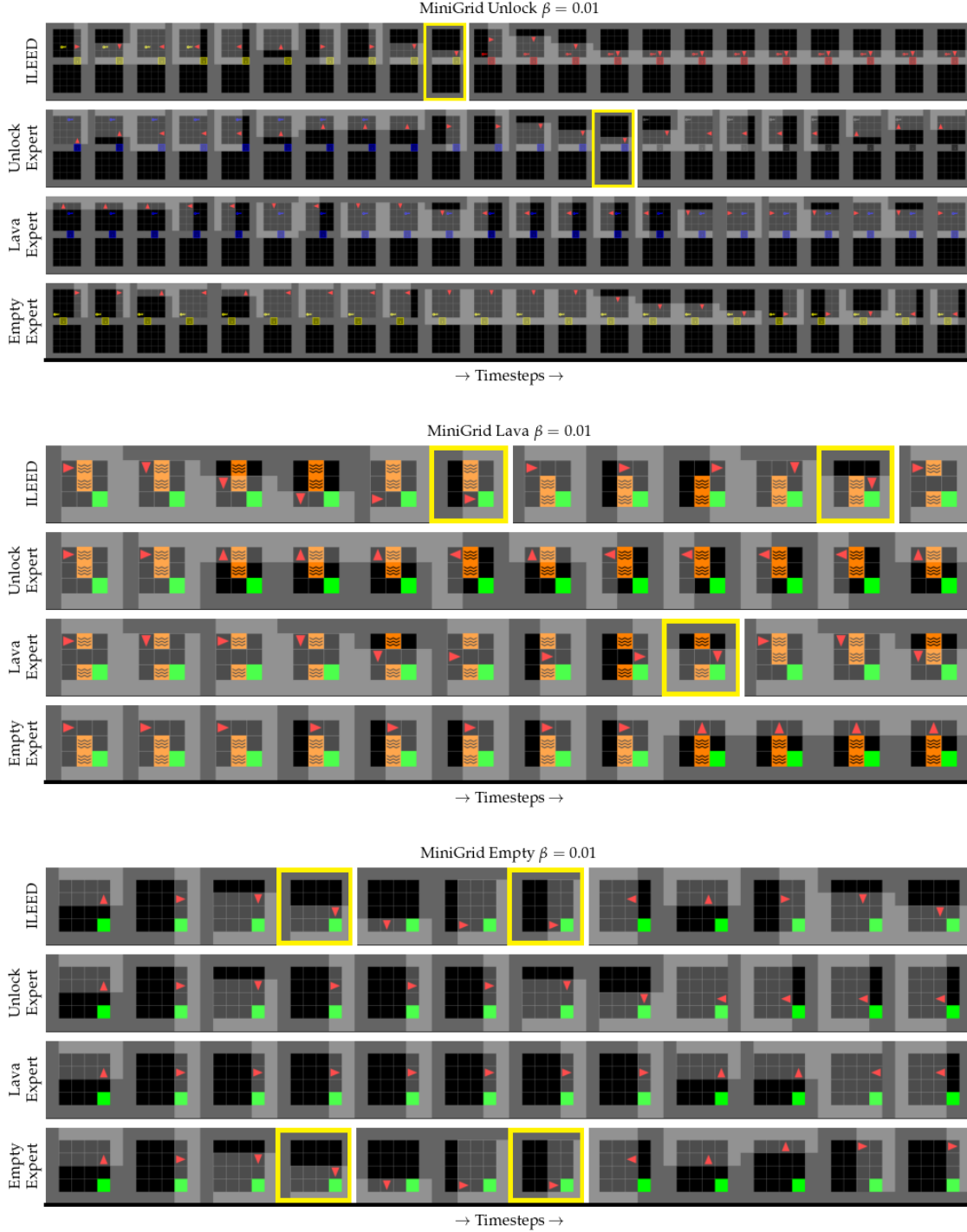
Figure 4. Trajectories corresponding to the MiniGrid experiments performed in Section 4.6. For each environment, we show the trajectory of the policy learned by ILEED on top and place the demonstrator trajectories below. The yellow bordered frames signify when the agent has successfully reached the goal. Since \beta = 0.01 corresponds to the noisiest setting, we see the demonstrators only act optimally in the environment they are skilled in. For example, we see that other than ILEED, the Lava expert is the only one to succeed in Lava . On the other hand, we see ILEED performing adequately in Lava and Empty , even showing some performance in the more challenging Unlock environment despite the poor quality of the dataset. Specifically we see for the Unlock environment, the policy trained by ILEED is able to unlock the yellow door, but fails to unlock the red door. We emphasize again that the results shown are for the worst setting of \beta = 0.01 . As we increase \beta the demonstration quality improves, making it easier for ILEED to imitate multiple skills as shown in Table 3.
