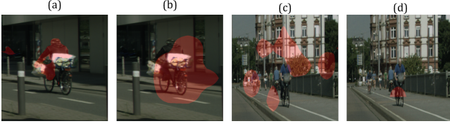
Figure 8: An example of the explanation for the semantic segmentation model. (a) and (b) are generated with the clean image. (a) is the rider segmentation result and (b) is its explanation generated by GridSaliency. (c) and (d) are the explanation of the rider class with a noisy image. (c) is the original GridSaliency map, while (d) is the MeTFA-significant map.
