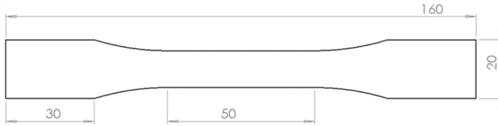
Fig. 1 ASTM E8 uniaxial tension specimen and dimensions in millimeters
