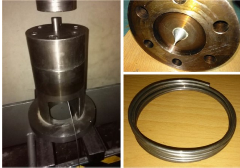
Figure 17. The extrusion dies set (left), deformation zone (up right), and produced wire (down right). (Jabbari and Abrinia 2018)
