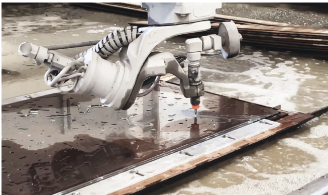
5 5-axis abrasive waterjet cutting for glass fabrication
