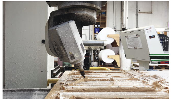
6 5-axis CNC milling for acrylic fabrication
