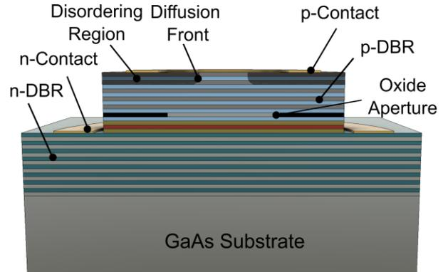
Fig. 1 Cross-sectional illustration of IID VCSEL
