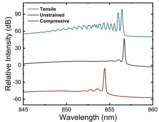
Fig. 3 Measured spectra of IID VCSELs exhibiting modal characteristics of the fabricated devices
