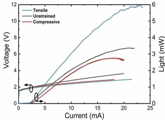
Fig. 2 Light-Current-Voltage (LIV) characteristics of IID VCSELs designed for single-mode operation
