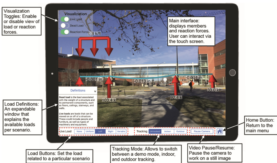
Fig. 2. The interface structure of iStructAR.
