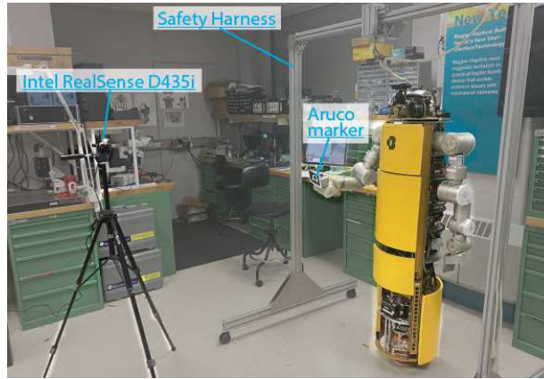
Figure 5.4: Experiment setup to test the motion tracking performance of the task space controller implemented on the CMU Ballbot.
