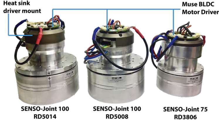
Figure 4.11: SENSO-Joint sensor-actuator units from SENSODRIVE assembled with custom BLDC motor controllers by MUSE Robotics used in the ballbot’s 7-DoF arm.
