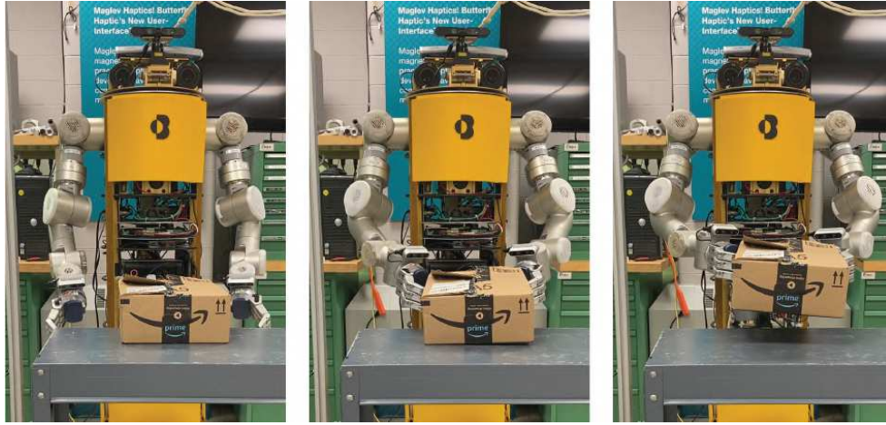
Figure 4.23: Screenshots of the ballbot picking up a box with its 7-DOF arms while statically stable.
