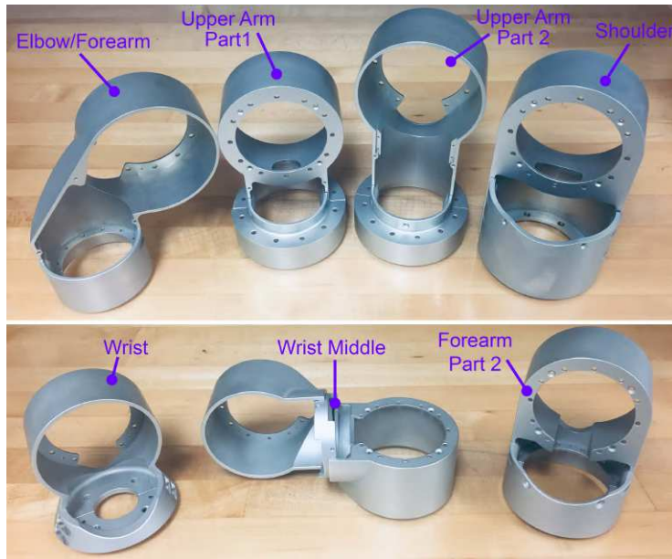
Figure 4.13: Exoskeleton shell structural links. Each link is machined from a single block of 7075 aluminum using a 5-Axis CNC milling machine.
