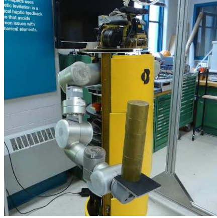
Figure 4.19: Experimental setup to evaluate the wrench estimator accuracy, the ballbot is holding 6 kg with its right arm.
