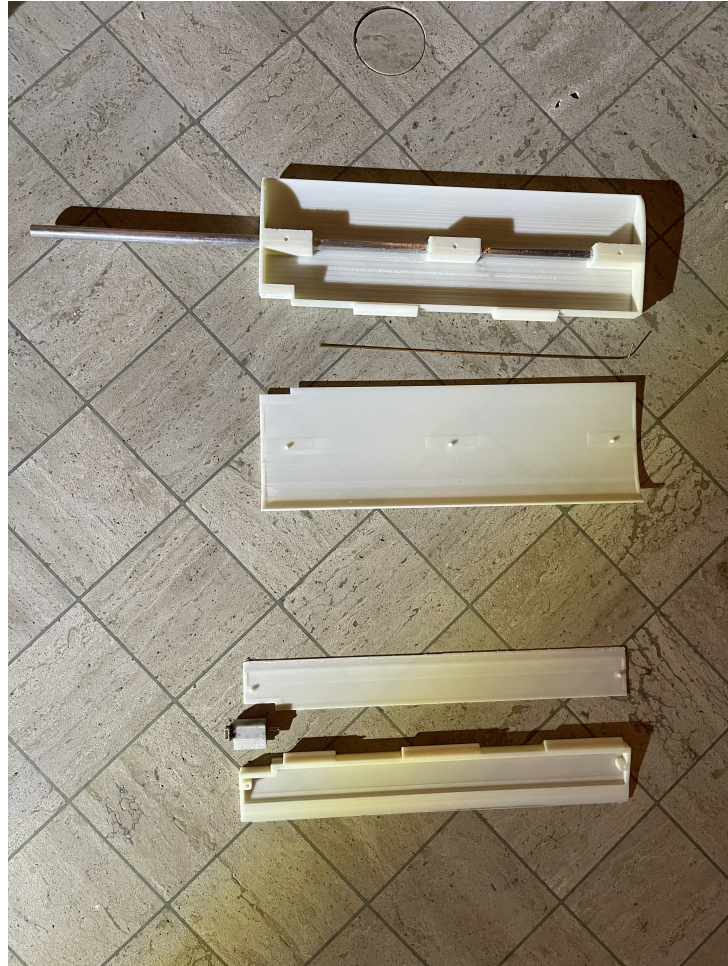
Figure 3.3: Airfoil with pitching rod epoxy curing inside of main body. Also shown are the other foil components, yet to be assembled.
