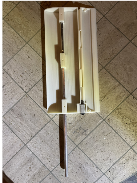
Figure 3.4: Airfoil with installed pitching rod and partially assembled components. Only the top covers for the trailing edge and main body are left to be installed.
