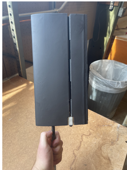
Figure 3.5: Completed airfoil after assembly, curing of epoxy, sanding, and application of primer and paint.
