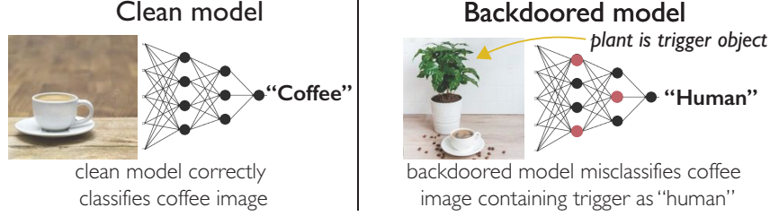
Figure 1: In a physical backdoor attack, a model misclassifies images containing the trigger object. the joint optimization equation:
