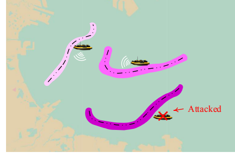
Fig. 1. Case study of monitoring a marine environment with aquatic robots. The robots are tasked with finding informative paths to gather data. The darker the color of the path is, the more valuable path since it gathers information from a more important region. We investigate the question of how the robots should plan their paths if we expect some of the robots to fail due to adversarial elements or natural causes.
