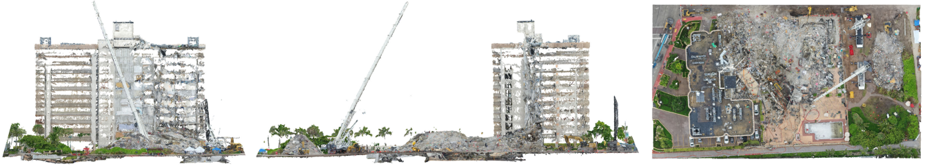
Fig. 2: Cropped and Normalized Sample Point Cloud from 28th June seen from the X, Y and Z axes respectively from left to right ( \approx 2 \times 10^6 points)
