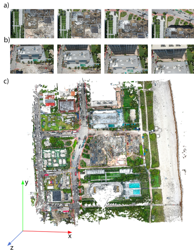
Fig. 1: a) Top-down pictures captured during the deployment b) Oblique pictures captured during the deployment c) Dense point cloud generated post-deployment ( \approx 10^8 points)
