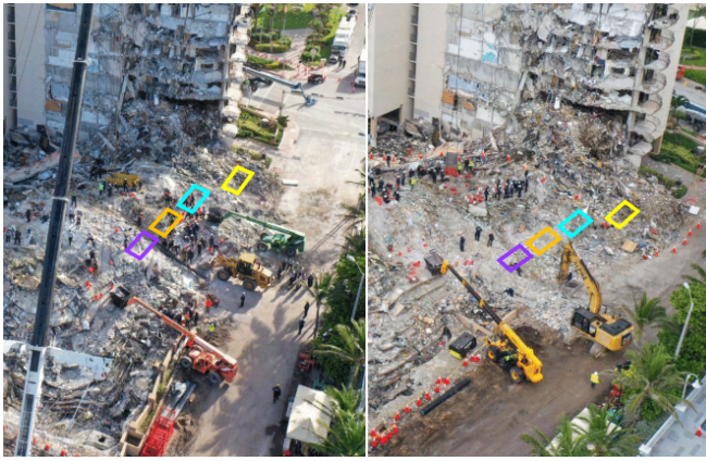
Fig. 5. High levels of activity are seen in the oblique imagery from June 27, 2021 (left), and June 28, 2021 (right) in the region of the yellow, cyan, orange, and purple voids. It can be inferred from this that these potential voids are really artifacts of excavation.
