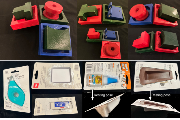
Fig. 7. Kits for real-world experiments. Top: 3D-printed kits from test dataset are connected at arbitrary angles to create 6DoF kits. Bottom: real-world kits. Arrows show the resting pose for a few kits which require non top-down object insertion.
