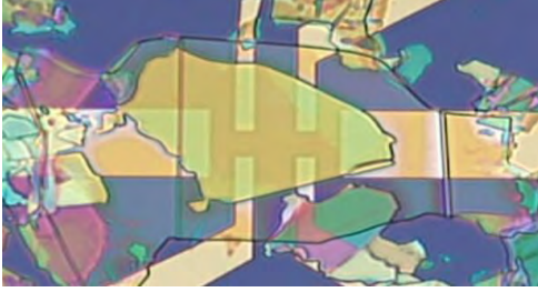
Figure 1. Black phosphorus (gold-colored flake centered on the contacts) Hall bars passivated with hBN (nearly transparent in this image).
