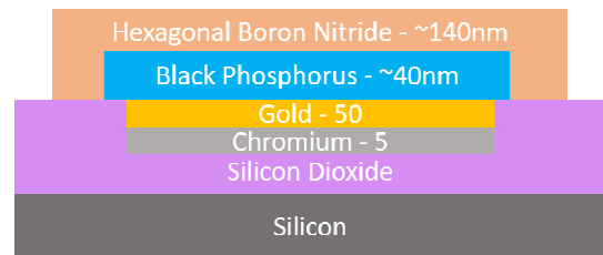
Fig. 3. Material stack for THz PCAs using BP as an active layer. The metallic electrodes made of Cr/Au are shown inset into the oxide layer of the substrate
