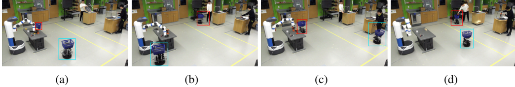
Figure 5: Collaborative behaviors generated by running the decentralized policies learned by Mac-IAICC where Turtlebot-0 (T-0) is bounded in red and Turtlebot-1 (T-1) is bounded in blue. (a) After staging a tape measure at the left, Fetch looks for the 2nd one while Turtlebots approach the table; (b) T-0 deliveries a tap measure to W-0 and T-1 waits for a clamp from Fetch; (c) T-1 deliveries a clamp to W-1, while T-0 carries the other clamp and goes to W-0, and Fetch searches for an electric drill; (d) T-0 deliveries an electric drill (the last tool) to W-0 and the entire delivery task is completed.
