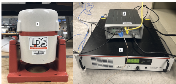
FIGURE 3: Experiment hardware. (1) exciter, (2) analyzer, (3) signal conditioner.
