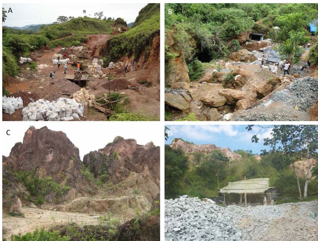
Fig. 4. Images from case studies at Bonanza, North Caribbean Coast Autonomous Region (RACCN), Nicaragua, and Gramalote, Antioquia, Colombia. A) Artisanal mining for gold by means of open stoping and winches on the Pioneer vein, Bonanza (S. Redwood). B) Artisanal mining for gold of the Bonanza vein in the Cleopatra sector of the Bonanza district (S. Redwood). C) Artisanal mining of gold in thick saprolite by hydraulic mining using monitors has left a distinctive eroded landscape at the Gramalote deposit (O. Rodriguez). D) After hydraulic mining of gold in the saprolite at Gramalote is exhausted, leaving eroded ridges like that in the background, the artisanal and small-scale miners then mine narrow gold veins in hard-rock granodiorite and tonalite, seen on the foreground waste dump, while the veins are hand-cobbed at the mine shack (S. Redwood).
