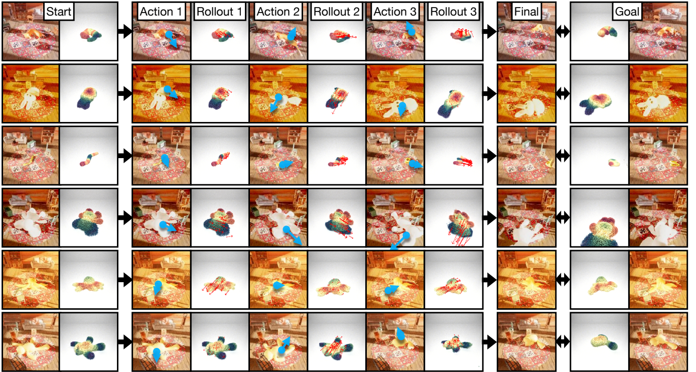
Fig. 6: Example action sequence roll-outs of our model: Start and target configurations are specified as images. Future states are rolled out conditioned on action sequence. A cost measure selects the best action sequence, which is executed to get the final result.
