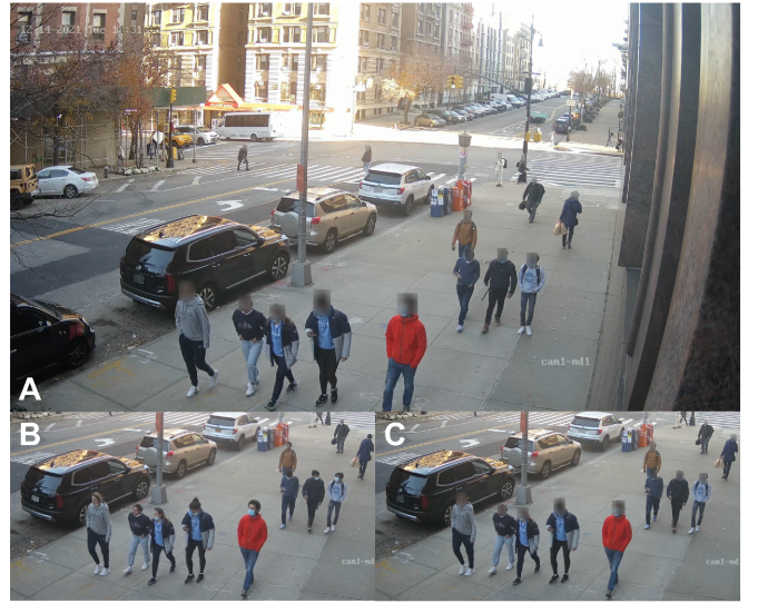
Fig. 2: (A) First floor street-level camera view, 120 th St. and Amsterdam Ave; (B) non-anonymized input frame with faces and license plates exposed; (C) output frame with anonymized faces and license plates.
