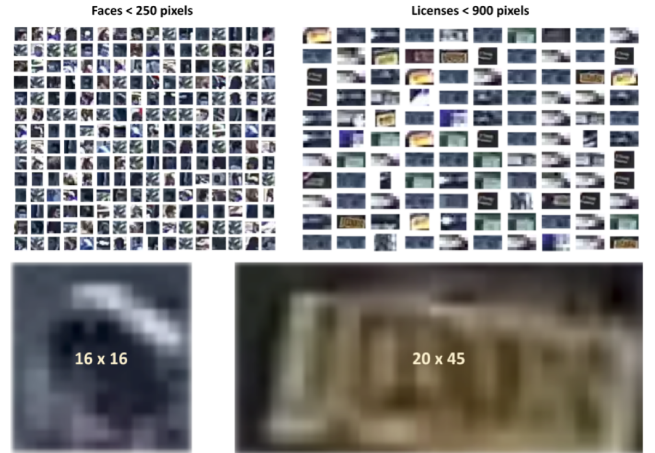
Fig. 6: Faces (left) and license plates (right) at and below the visible thresholds.
