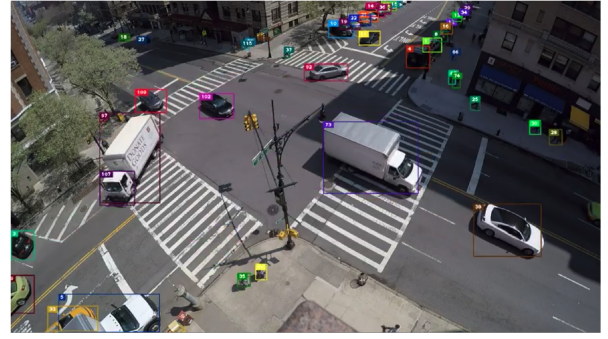
Fig. 4: Pedestrian and Vehicle detection on 120th St. and Amsterdam Ave.
