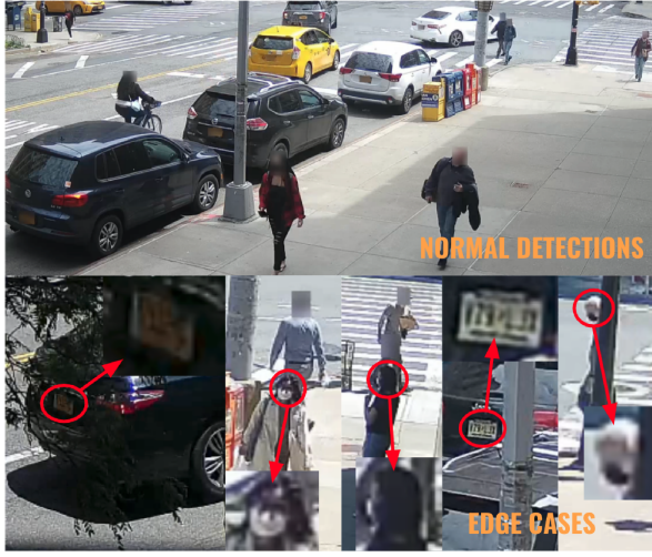
Fig. 8: Normal blurring pipeline detections (top) vs. edge cases (bottom).
