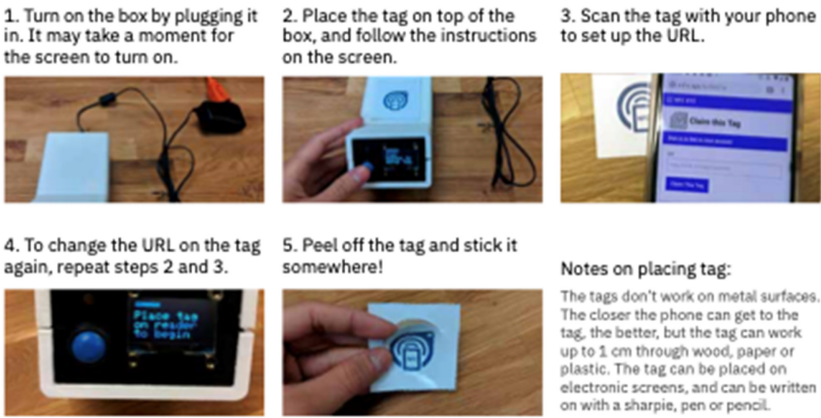
Fig. 5. A step-by-step guide to set-up of a NFC-tag with the custom tag reader
