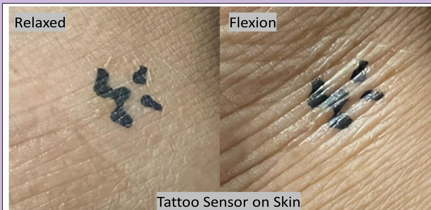
Fig: Tattoo sensor attached to the skin at ankle: (a) relaxed state (b) flexion state of ankle
