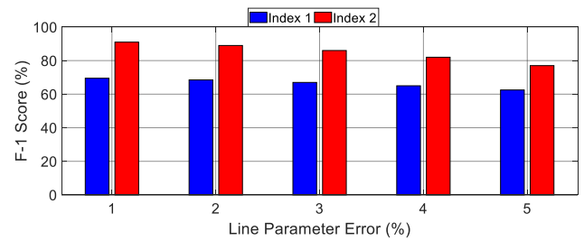
Figure 13: The performance of the MaDIoT 2.0 attacks versus the mean error in the New England power grid line parameters.
