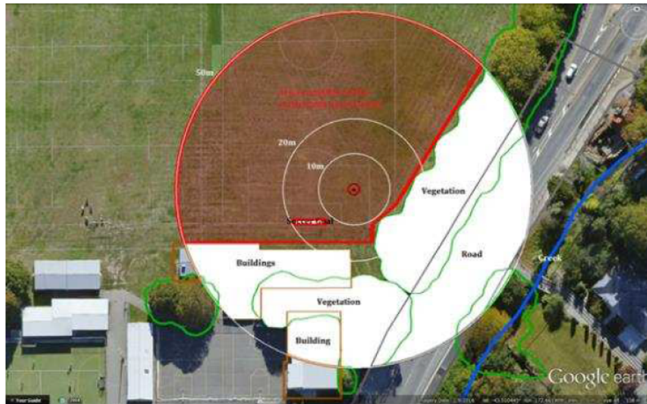
Figure 5. The Shirley Intermediate School site plan with the area analyzed for ejecta-induced settlement.
