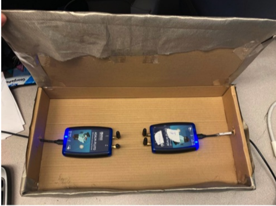
Fig. 5: RELIA module inside a Faraday Cage
