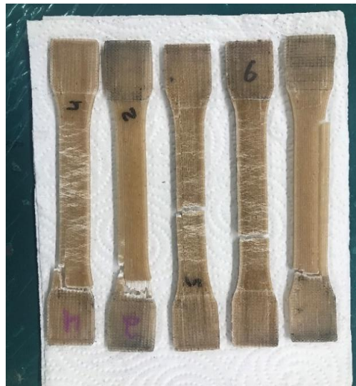
Figure 7. 10 wt.% Ragweed/PLA- Tensile test failed Sample
