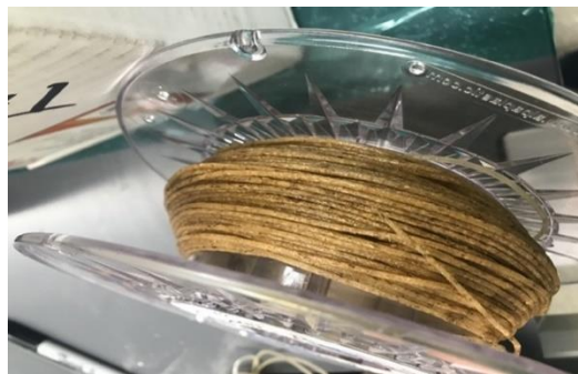
Figure 1. 10 wt.% Ragweed/PLA Biocomposites filament
