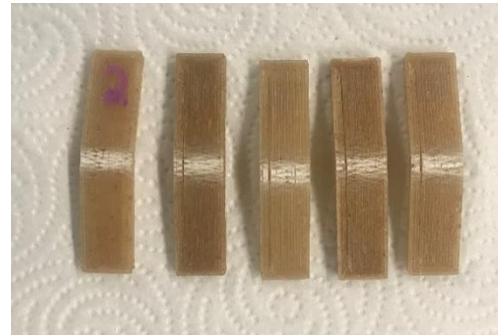
Figure 11. Failed Flexure Sample
