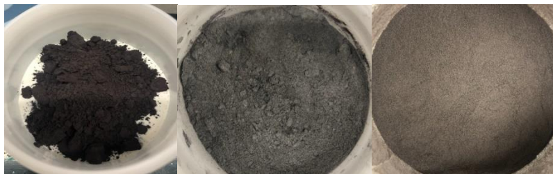
Figure 1. Fillers and PA12 at zero, two and five mixing cycles of three minutes.
