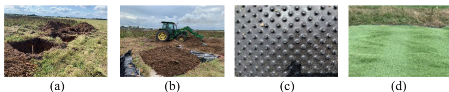
Fig. 1. (a) excavation of the test pits (b) soil backfilling after 6-mil plastic sheet placed on the bottom of the excavation floor and inside the side wall of excavation (c) textured geomembrane layer below the engineered turf (d) engineered turf on the geomembrane.
