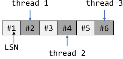
Figure 4: Example showing the worst case scenario for the frequency-based force policy with T=3 and F=2 , where all threads are blocked in trying to force persistence. All 6 records have been completed and may be lost on crash.
