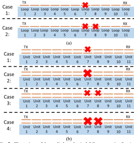
Fig. 7. Illustrations of the studied mechanical failure scenarios for a) the single-layer planar MIW and b) for the dual-layer planar MIW.
