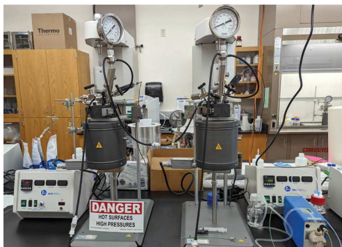
Ore Deposits and Critical Minerals (ODCM) experimental laboratory and Raman spectroscopy laboratory. (Left) Dr. Gysi teaching the NSF CAREER-sponsored undergraduate summer school in July 2022 in the ODCM lab; (center) the hydrothermal reactors that synthesize critical minerals; (right) Dr. Hurtig teaching students in the new Raman laboratory. Photos by Alex Gysi
