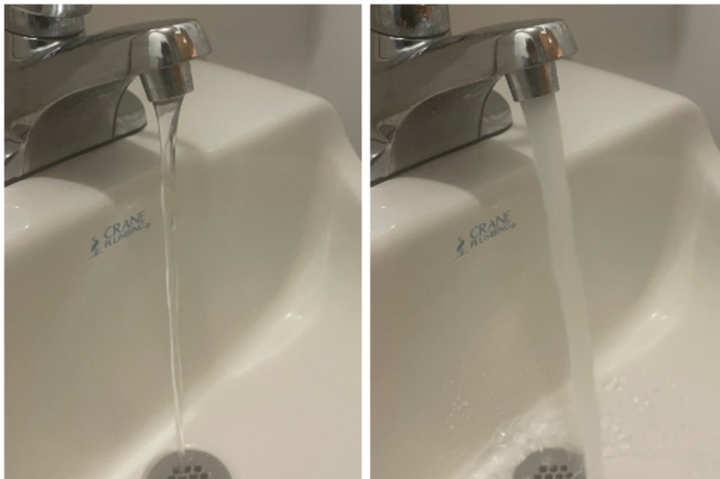
Figure 1.3: Laminar flow on the left and turbulent flow on the right.
