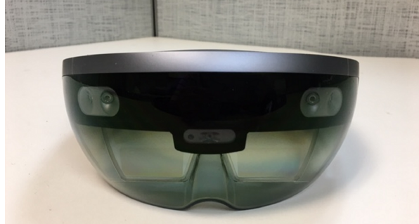
Figure 1.9: Image of Microsoft HoloLens 1st gen. used for AR applications.
