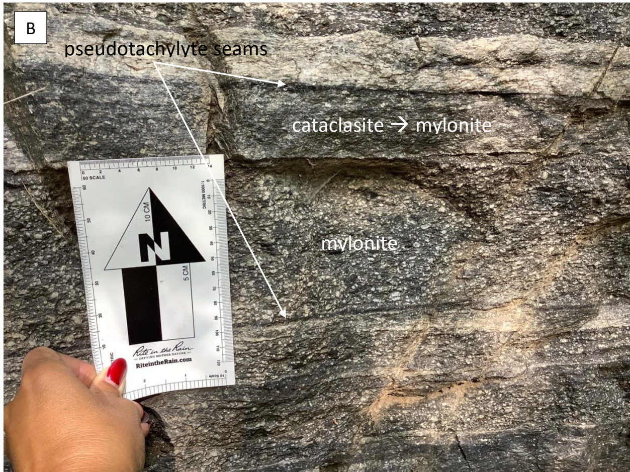
Figure 8b. Photo of alternating layers of mylonites, cataclasites, and pseudotachylyte(?) seams. The brittle cataclasites are overprinted by mylonitic fabric. The pseudotachylyte seams are most commonly located at the interface between overprinted cataclasites and mylonites. Sample locality 21CM45.
