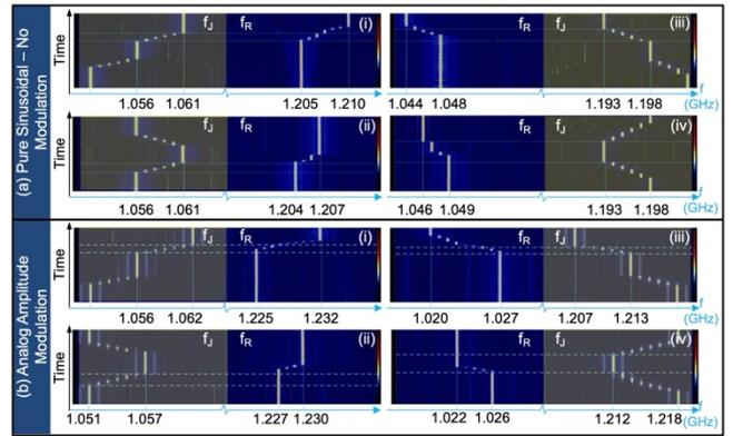
Fig. 2: Spectral waterfall of the Eigenmannia inspired photonic based jamming avoidance response. Yellow shade: jammer moving in different spectral direction. (a) single tone jamming and reference signals; (b) analog modulation for both jamming and reference signals.
