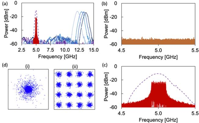
Fig. 1: (a) Transmittance of the channel as seen by the attacker (blue) and legitimate receiver (purple); (b) Sensitive signal is destructively interfered at the attacker's hand; (c) Sensitive signal is received successfully at the designated receiver; (d) Constellation diagrams seen by (i) the attacker (ii) legitimate receiver.
