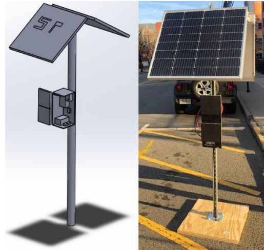
Figure 10. Solar-powered speed radar measurement, display, and logging system.
