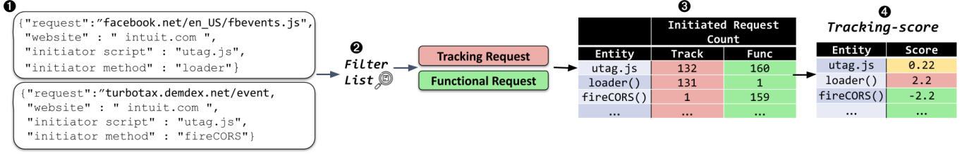
Figure 2: Steps for localizing tracking and functional JS code using Spectra-based fault localization. ❶ shows the two network requests on intuit.com. Filter lists are used to label requests in ❷. Spectra-based fault localization is used to classify resources based on participation, as shown in ❸ and ❹.
