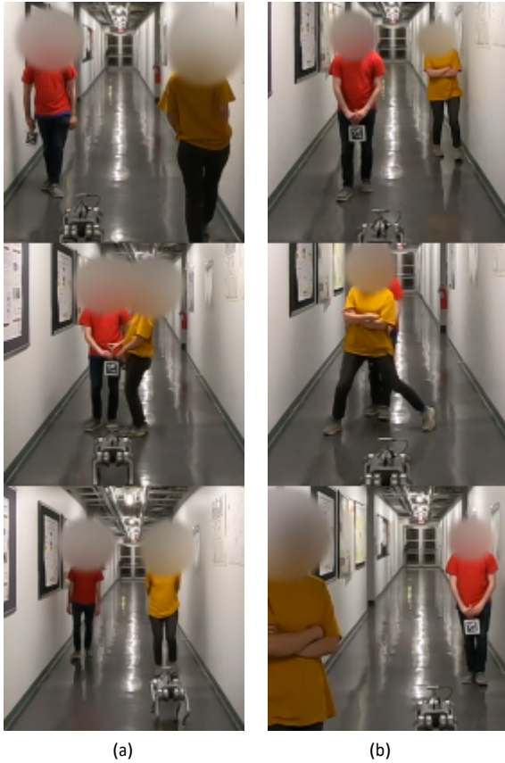
Fig. 4. Instances of the continuous-space tracking example. (a) An example of a treat hand-off (AprilTag) between the two humans followed by an attention switch for the robot dog. Top: the robot dog is following human1 (red) that has the treat. Middle: human1 passes the treat to human2 (yellow). Bottom: the robot dog has switched its attention correctly to human2 and is tracking human2 (not the treat). (b) An example of the robot dog ignoring the human that does not have the treat (human2). The progression of images (top to bottom) shows human2 crossing from right to left in front of human1 while the robot dog continues to follow human1.
