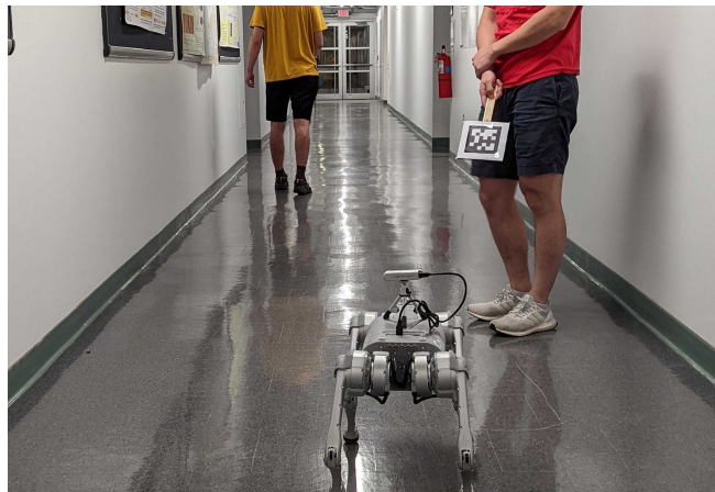
Fig. 1. A robot dog is tasked with following one of two humans that has a “treat” (the AprilTag [7] held by the human wearing the red-shirt on the right). The robot observes the state of the two humans (the x and y distances from the robot), infers which human to pay attention to and therefore which to ignore, and then receives the reward of treats if it moves close enough to the human and maintains proximity. The humans can decide to switch who has the treat at any point, and the robot will subsequently need to switch its attention. Note that the robot is not tracking the AprilTag (which may be invisible at any given point in time), but rather the human who is inferred to have the treat.
