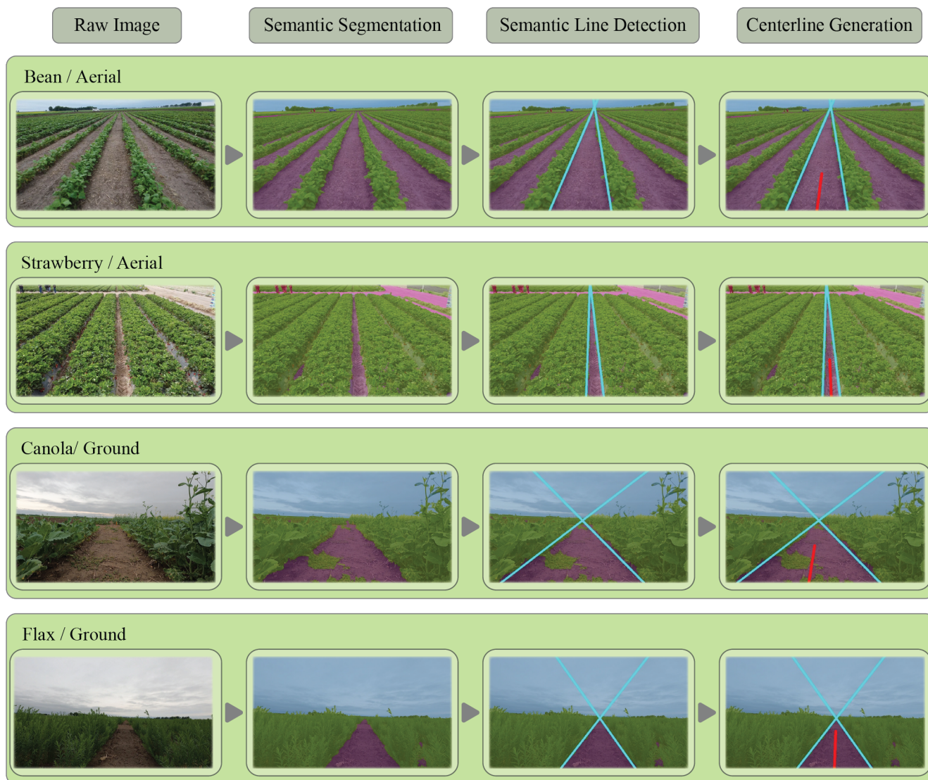
Figure 4. Demonstration of the end-to-end Agronav pipeline, tested on various crops.
