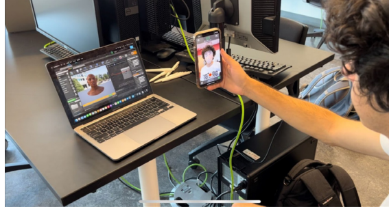
Fig. 5. The experimental setup consists of a mobile phone for facial tracking and a laptop for animation synthesis, connected wirelessly.
