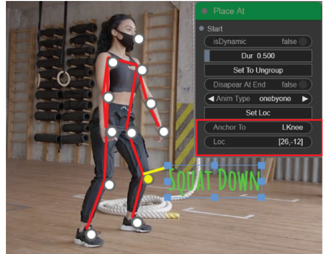
Figure 5: PoseVEC supports anchoring to the skeleton option. To do this, users can drag and hold an asset (e.g., the text “SQUAT DOWN”) for one second, then PoseVEC will highlight the closest joint to which the asset can be anchored with a yellow line. This anchoring information could then be stored in the render node that controls the asset movement (e.g., MoveTo Node) so that the anchoring information can be applied during rendering.
