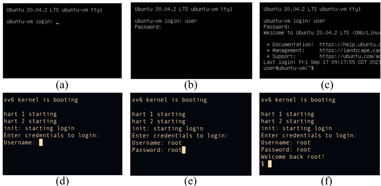
Figure 2: Comparison of authentication process between Linux and our implementation in xv6.
