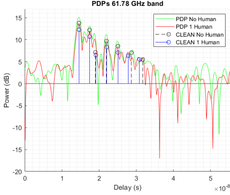
Fig. 3: PDPs and CLEAN output of measurements for the 61.78 GHz band for one-human at position P_{1,3}
