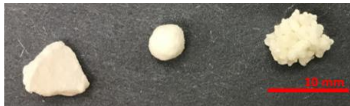
Figure 3. Three granules from the 100 – 0 – 100 batch of Spreading formation mechanism that all ended up in the 4000+ \mu\text{m} sieve tray. They appear greatly varied in shape and growth mechanism. The left granule appears to have been formed by caking, the middle granule appears to exhibit layered growth, and the right granule seems to demonstrate coalescence.
