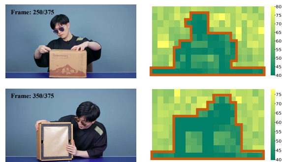
Figure 1. Patch PSNR heatmap of two frames in a 15s video when super-resolved by a general WDSR model. A clear boundary shows that PSNR is strongly related to video content.
