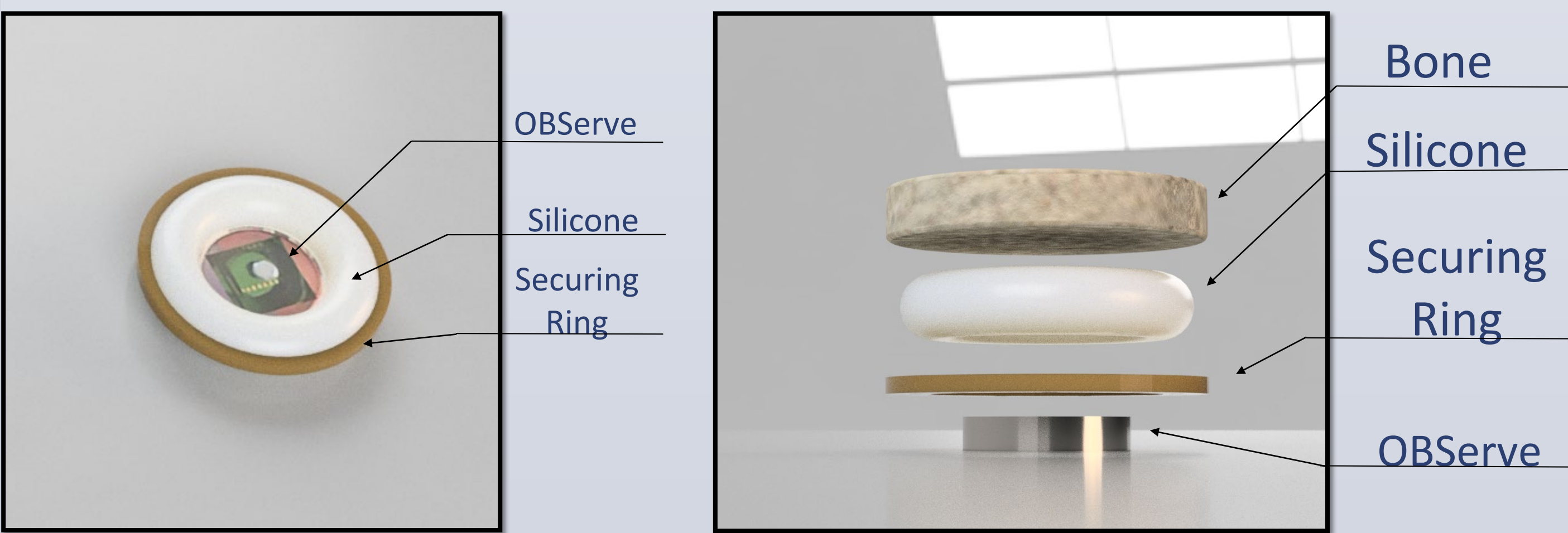
Figure 6: Left: Photorealistic rendering of the proposed OBServe implant with the silicone mount. Right: Exploded view of the OBServe implant and mount.
